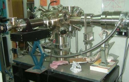
Scanning tunneling microscope
